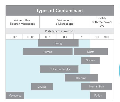
Contaminants that pass through an industry-standard 5-micron filter
